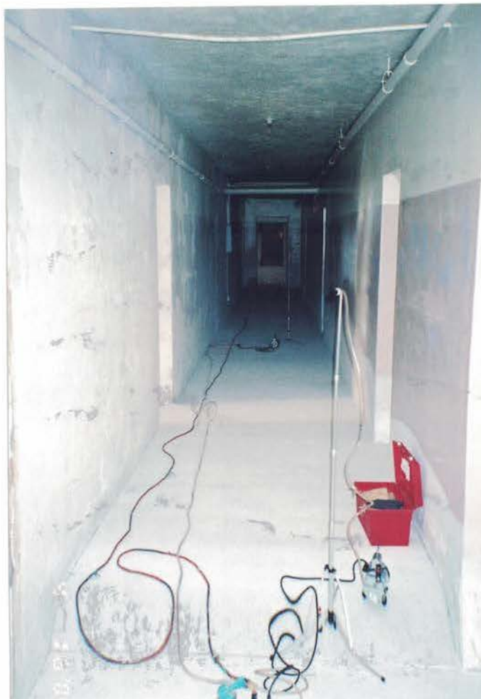
Photo #49: Post-abatement air sample 09TEC104-19, collected in the central portion of the 1st floor near the main entry, is reported with an airborne count of < 17 str/mm 2 of asbestos which is well below the AHERA clearance standard of < 70 str/mm 2 . Note the thorough layer of encapsulant on the concrete floor following the removal of asbestos-containing vinyl floor tile and black mastic. Viewing northwest.
