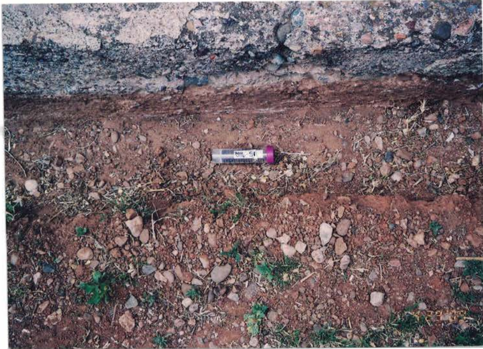
Photo #53: Composite soil sample B116-51, collected from topsoil following the removal of lead-contaminated soil surrounding the building, is reported with a lead count of 140 ppm which is below the HUD clearance standard of 400 ppm for bare soil. Spray removed topsoil to a depth of 6-inches in a 6 foot radius around the perimeter of the building. Viewing down.
