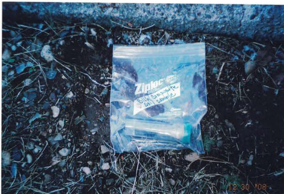
Photo #10: Composite soil sample B116-02L was collected from the perimeter of the building to determine if the soil surrounding the dormitory is contaminated with lead. Soil sample -02L is reported with 5,300 milligrams per kilogram (mg/kg), or parts per million (ppm), which exceeds the HUD clearance level of 400 ppm for bare soil. Viewing down.
